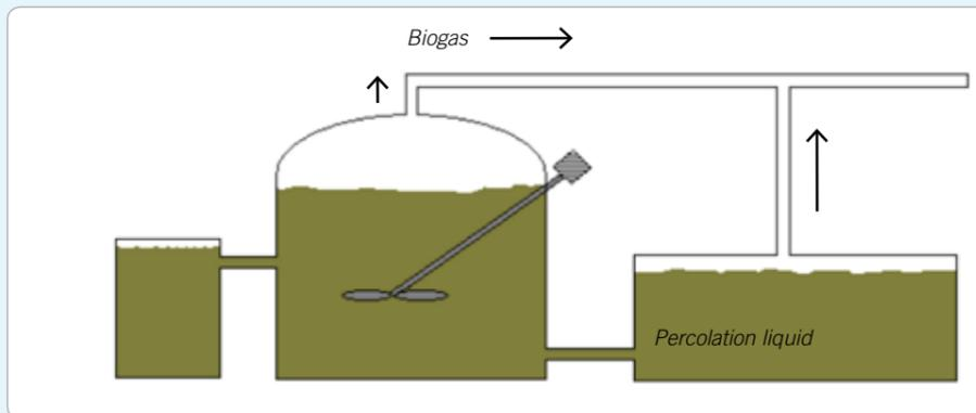
Concept of a wet digestion facility with propeller agitation and continuous operation.
