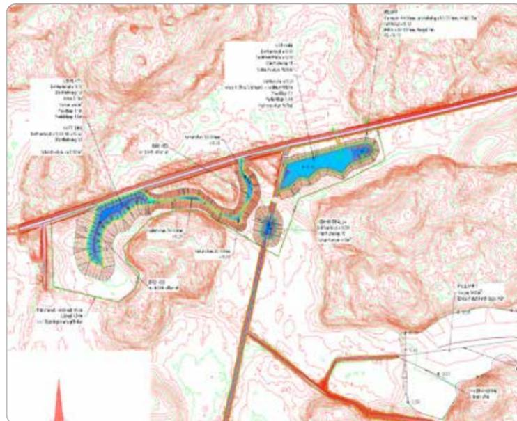
Example of plans and actions along the Gris creek: wetland with a new side branch, a sediment trap and a fish habitat.
